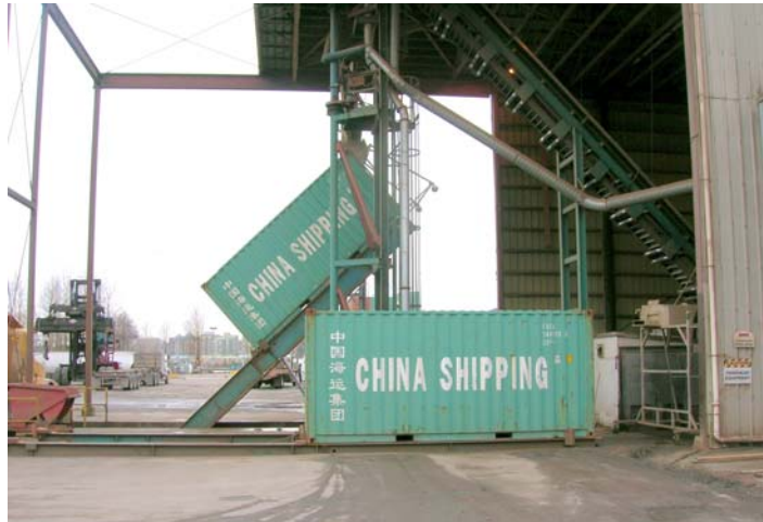
Figure 10 – Port Transloading of Bulk grain (WestNav, Vancouver)
